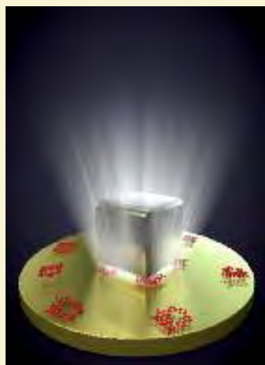
This illustration created by Gleb Akselrod, a postdoc in electrical and computer engineering, depicts a silver nanocube and gold film sandwiching fluorescent molecules (red) to speed up their fluorescence.
