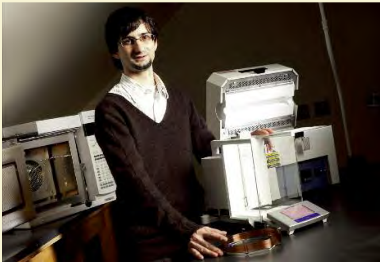
Nico Hotz, assistant professor of mechanical engineering and materials science at Duke, stands with a catalytic prototype that produces hydrogen by reforming fuel at much lower temperatures than conventional methods.
